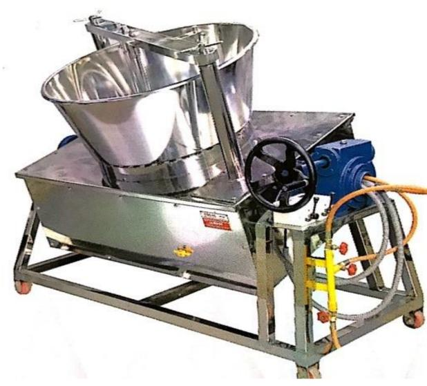
Scope of supply; Stainless Steel heavy duty body structure, **with tilting attachment** v-belt type mechanism, Ceramic coating high pressure Gas Burner, with 0.5 H.P. motor Blower, 1.0 H.P. Electric Motor, and Double pillar scraper attachment.
