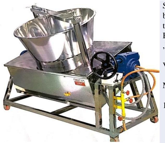
Scope of supply; Stainless Steel heavy duty body structure, with tilting attachment v-belt type mechanism, Ceramic coating Gas operated Burner, (without blower ), with 1.0 H.P. motor, Double pillar scraper attachment.
