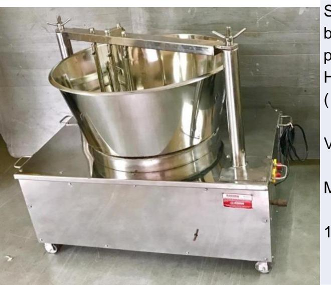
Scope of supply; Stainless Steel heavy duty body structure, Ceramic coating high pressure Gas operated Burner, with 1.0 H.P.+ 0.5 H.P motor Blower Electric Motor, (without diesel tank)
