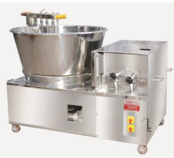
Scope of supply; Stainless Steel heavy duty body structure, v-belt type mechanism,
